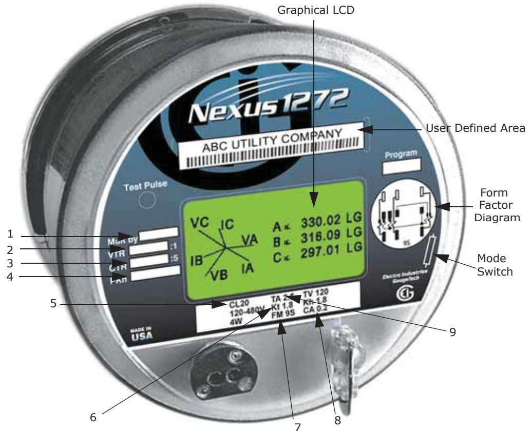
Figure 3.1: Meter Showing Faceplate Elements
