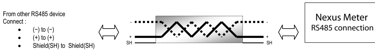
Figure 4.4: 2-Wire RS485 Port Detail
