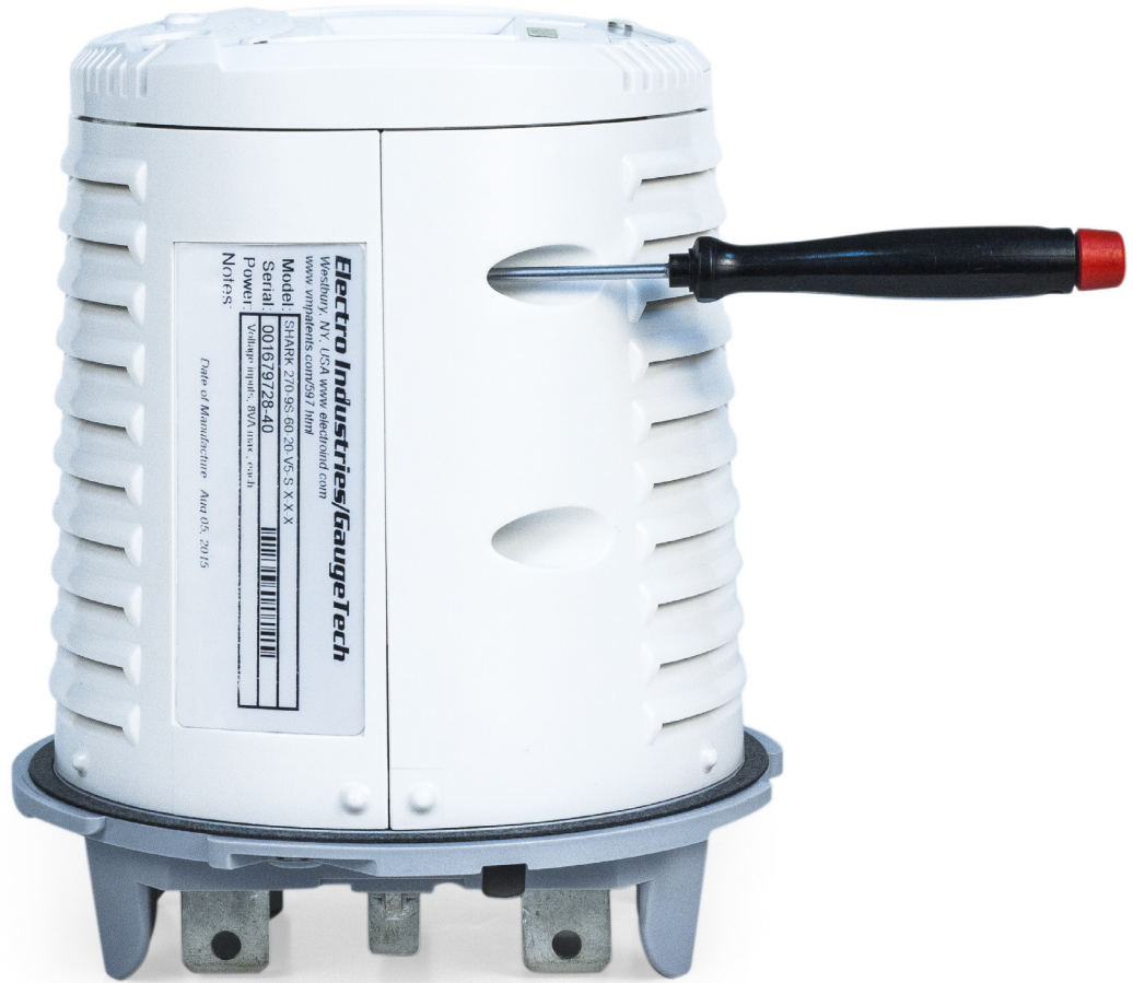
Figure 8.10: Separating Cover Halves
