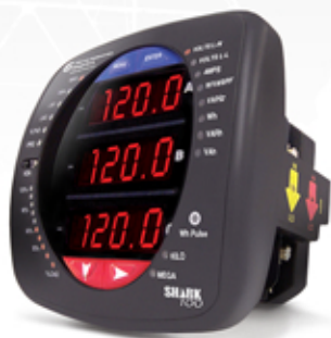
SHARK ® 100 Multifunction Meter 0.2% Class with Modbus + DNP 3.0
